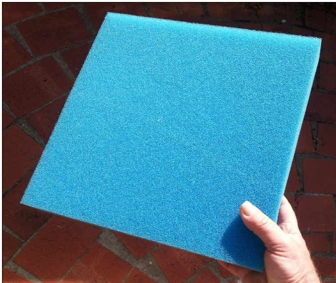
Photo 2: A precut 33cm x 33 cm x 5cm thick block of Poret 30 PPI foam ready to use as a filter or divider. The blue colour seems to be “traditional” and easiest to find but it does come in a variety of colours.
